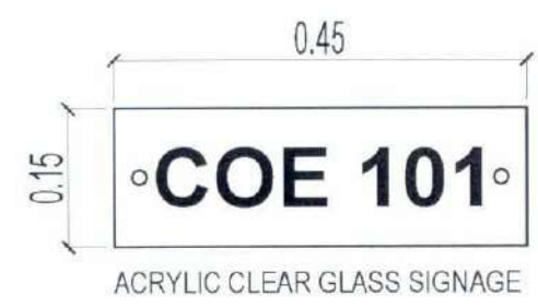
TYPICAL ROOM SIGNAGE DETAIL SCALE 1:10MTS.
